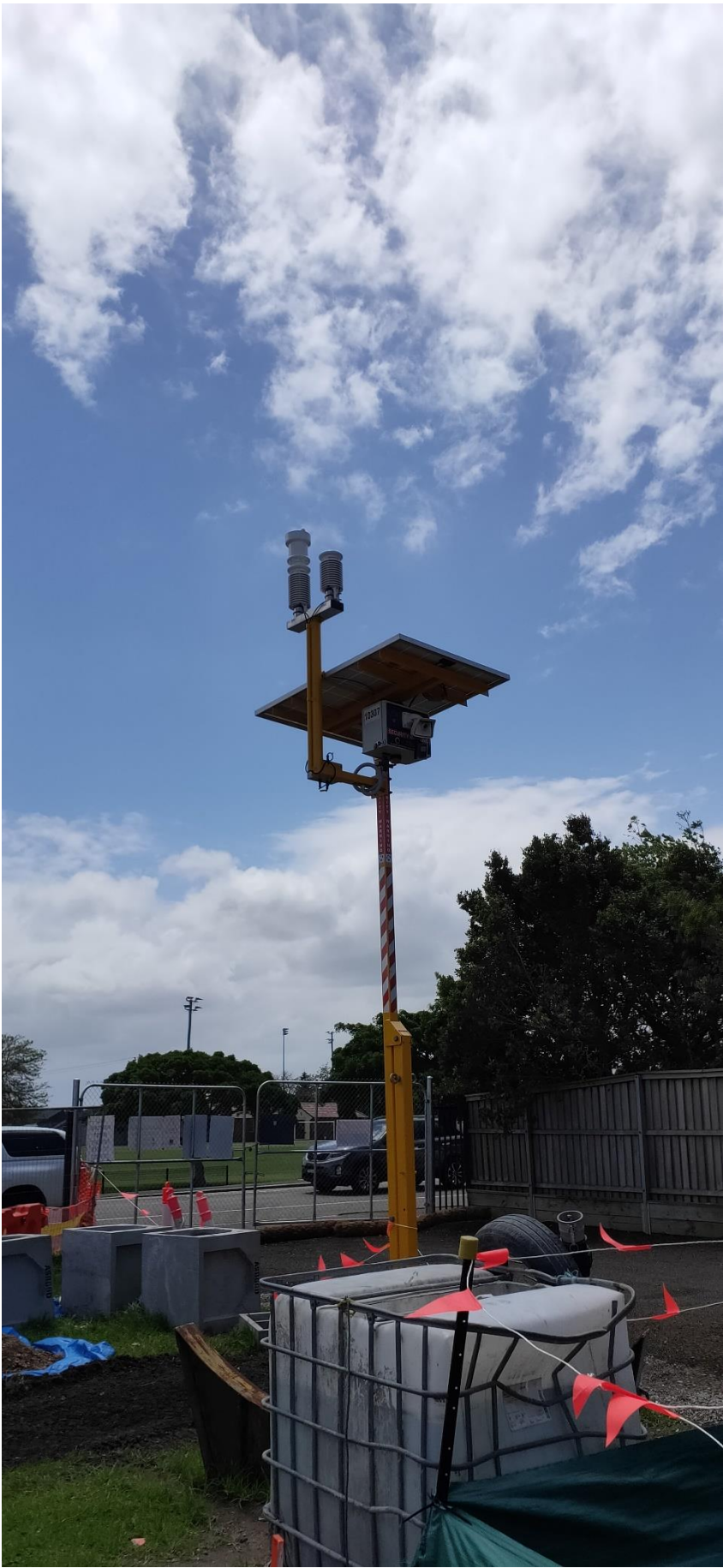
Photograph C.9 Real time noise and weather monitoring
